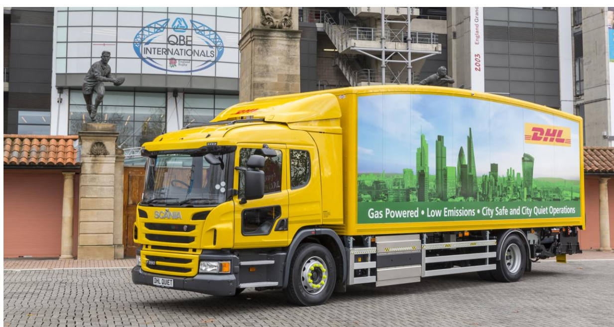
Figure 4. A currently available OEM dedicated gas rigid vehicle
